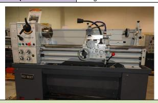
**Potential Hazards:** High power rotating spindle with exposed moving parts can cause entanglement, impact, flying debris and electrical hazard with the potential to cause serious harm and/or even death. Exposure to heat, noise, projectiles and sharp objects.
