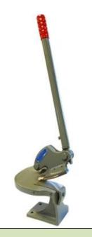
**Potential Hazards:** Exposed blade with significant mechanical advantage when handle is pulled. Exposed moving parts and gears. Extreme cutting hazard is always present. Risk of cuts from sharp work piece edges after every cut.
